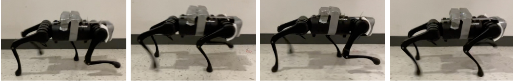
Figure 5: Trotting with 1 kg payload (two bottles of 500 ml water are strapped onto the robot). The 1 kg payload is out of the normal perturbation of environment parameters used in simulation training shown in Table 1. We show qualitative and gait patterns for other two gaits in the appendix. We find that the gait patterns are robust and remain the same even in the presence of disturbances.
